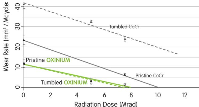
Plot of the mean wear rates ( $\pm$  standard deviations) in a knee simulator for UHMWPE crosslinked to various doses against either CoCr or OXINIUM femoral components in pristine (solid symbols and lines) and tumbled (open symbols and dashed lines) conditions.
