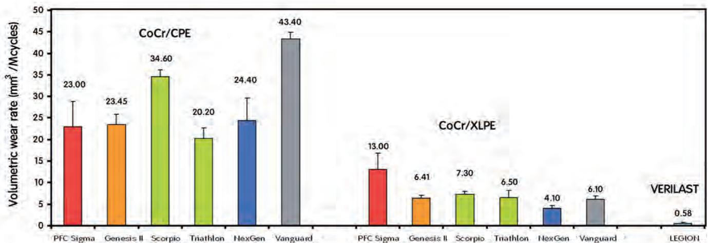
Mean volumetric wear rates (+/- std. dev.) of CoCr against conventional polyethylene (CPE), CoCr against crosslinked polyethylene (XLPE) and OXINIUM against XLPE (VERILAST) [30-36].
