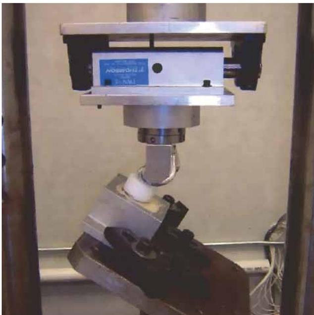
Photograph of the set-up for lock-strength and fatigue tests of posterior-stabilized (PS) tibial inserts.
