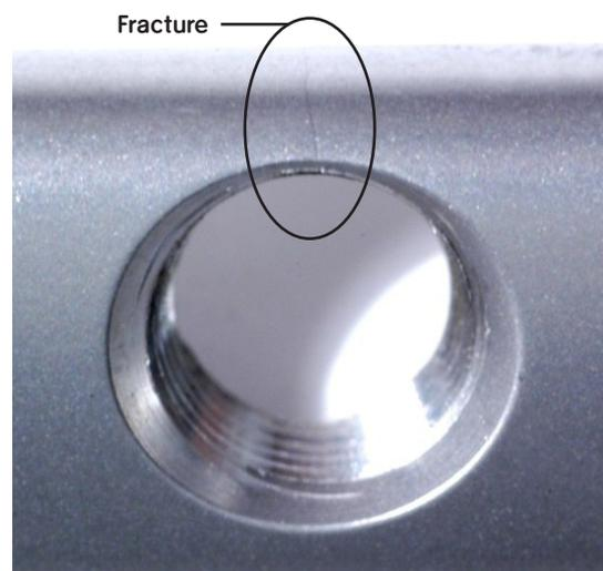
Typical Fracture of the SS PERI-LOC Locking Compression Plate with and without locking screw hole fillers (4.5mm plate shown here).
