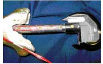
Figure 4 - Location of the strain gages on the femoral stem
