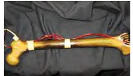
Figure 5 - LEGION Revision Knee femoral component and stem implanted in a composite bone
